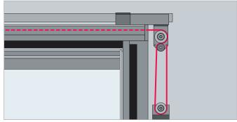
Simplified wire cable guide for the closing weight for easy installation.
