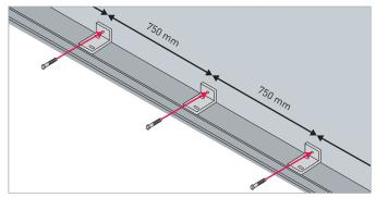
Easy installation due to single bracket mounting with extended 750 mm spacings, in the closing and parking area. Easy tolerance compensation during installation using long holes in the brackets and the track.
