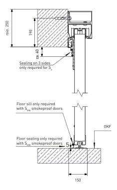
Door overlap 190 Clear passage ca. 10 Front side (running in) Sealing on 3 sides only required for S<sub>a</sub>
