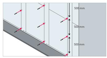
Panels connected to each other with 1-sided screw connection on the non-visible wall side (500 mm screw spacing).
