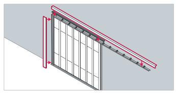
Simple screwless track cover as standard. Flush with counterweight casing.
