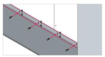
Quick and easy floor levelling via height-adjustable floorend profile.
