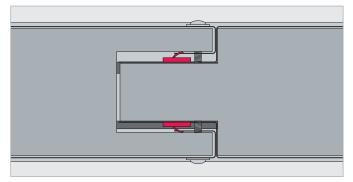
Integrated seals between the panel joints eliminates the need for on-site panel sealing with silicone for  $\rm S_a$  and  $\rm S_{200}^{}*.$
