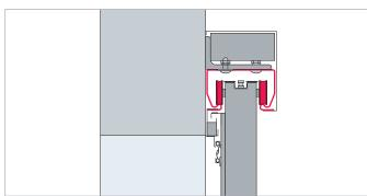
Special roller design compensates for unevenness in the wall and header areas.
