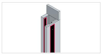
Reduced complexity due to factory pre-assembled elements including pre-mounted foam strips.
